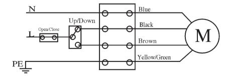
6. Check the UP and DOWN functions of the motor.
